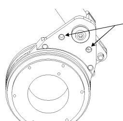
1/4" – 28 UNF holes for attachment of support brace(s).
