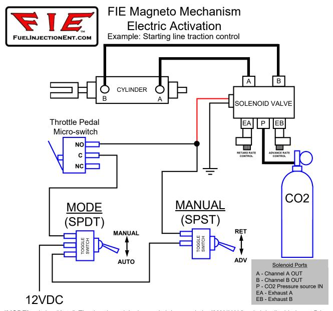
"MODE" switch = "Auto": The throttle pedal micro-switch is armed, the "MANUAL" switch is disabled, port B is active and the unit is retracted fully (retarded) against the zero stop. When the throttle pedal switch is activated, side B of the cylinder is exhausted and side A is charged, which moves the mag in the advanced direction until the cylinder reaches the stop.
