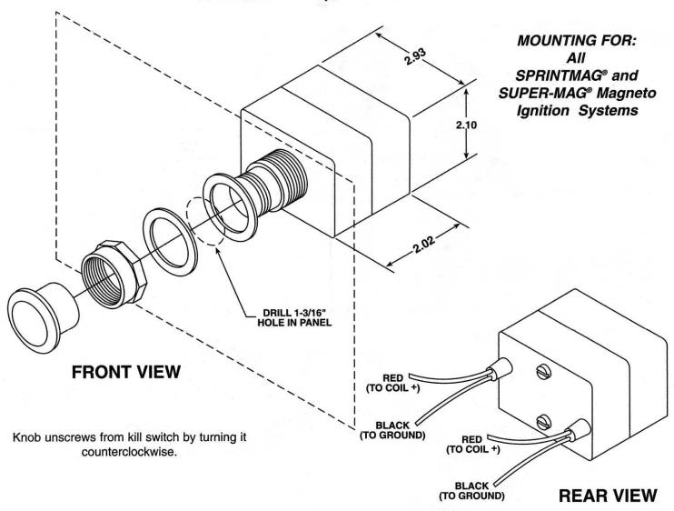
To kill the magneto ignition system, push the knob in. The knob locks in place. Turn the knob clockwise to release the lock. The internal contact area is sealed to prevent corrosion and the contact block is replaceable.
